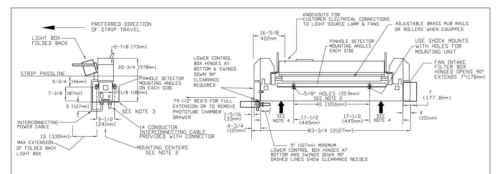
NOTE 2: MOUNTING HOLES INFORMATION 5/8 INCH HOLES ARE PROVIDED FOR MOUNTING THE PINHOLE DETECTOR ON 40 INCH X 9-1/2 INCH CENTERS. FOUR 1/2 INCH THREADED STUDS OR BOLTS CAN BE USED TO SECURE THE UNIT WITH PROVIDED RUBBER SHOCK MOUNTS.
